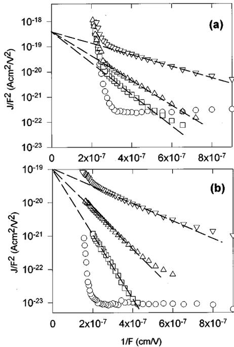
FIG. 1. Fowler-Nordheim plots of the dark (○) and the PST currents measured at photon energy 2.41 (□), 2.54 (△), and 2.71 eV (▽) in the MOS structures with SIMOX BOX produced by (a) single and (b) triple implantation. The PST currents are normalized to the incident light power of 1 W. The lines show the PST behavior expected from the FN model.
