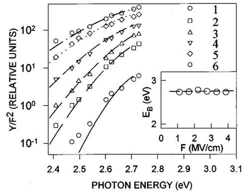
FIG. 2. Spectral dependences of the PST quantum yield in the SI SIMOX BOX taken at different strength of the electric field (in MV/cm): 1.1 (1), 1.67 (2), 2.22 (3), 2.75 (4), 3.33 (5), and 3.88 (6). The lines represent the FN model fitting results. The binding energy of the initial electron state of the PST transition  $E_B$  obtained from the fitting is shown in the insert as a function of electric field.
