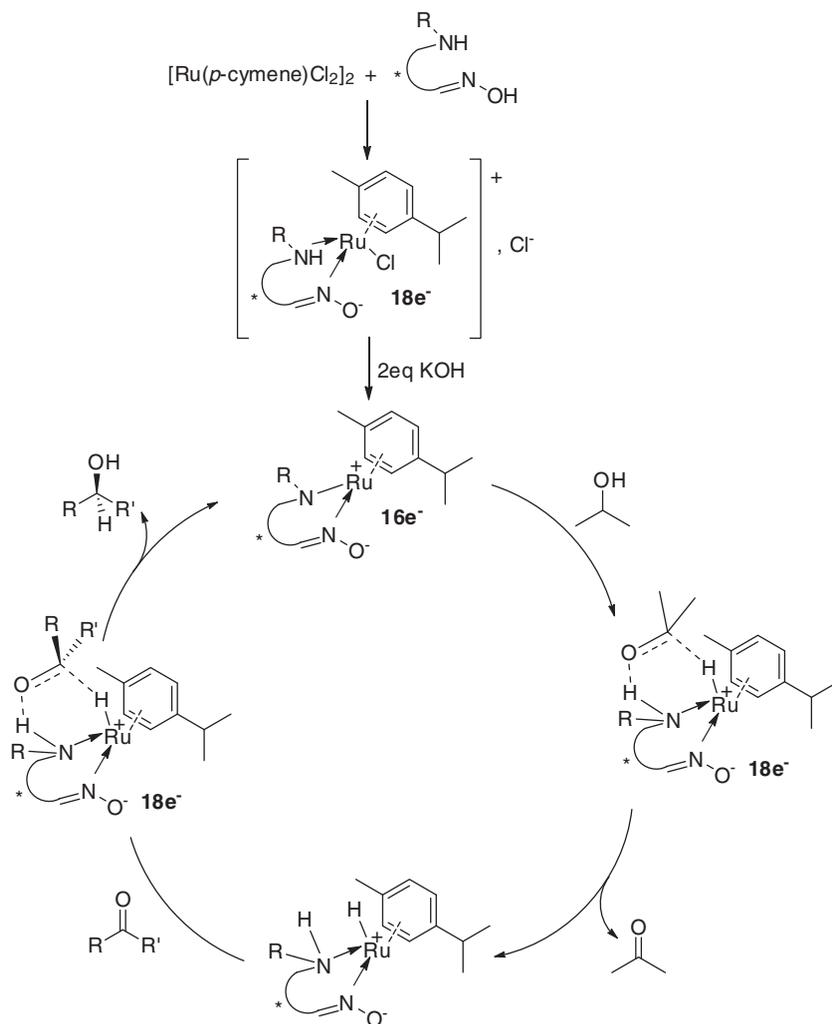
Fig. 4. Proposed mechanism for the asymmetric transfer reaction of ketones over Ru(arene)(aminoxime)-based catalysts.
