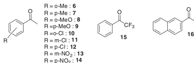
Scheme 4. Aromatic ketones used for asymmetric transfer hydrogenation.
