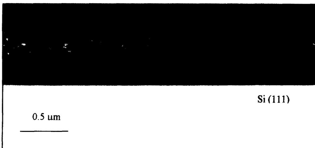
Fig. 1. (220) DF XTEM micrograph of the  $\text{SiO}_2$  layer, thermally grown on an Si(111) substrate, after  $\text{Si}^+$  ion implantation (160 keV;  $10 \mu\text{A cm}^{-2}$ ;  $1.2 \cdot 10^{18} \text{ cm}^{-2}$ ) and thermal annealing (1100 °C; 4 h).
