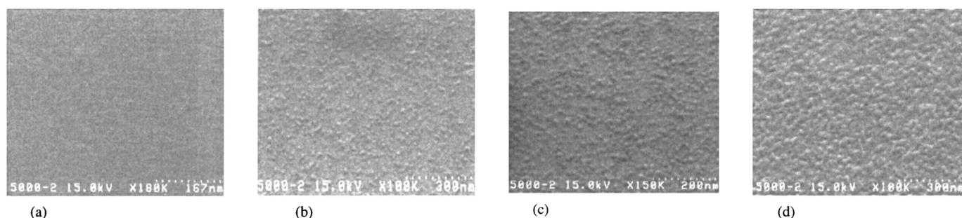
**Figure 2.** SEM images of dots deposited on the various growth times: (a) 60 s, (b) 90 s, (c) 120 s, and (d) 180 s at 520°C with 0.75 gas ratio of  $\text{GeH}_4$  to  $\text{Si}_2\text{H}_6$  on  $\text{SiO}_2$  substrate.
