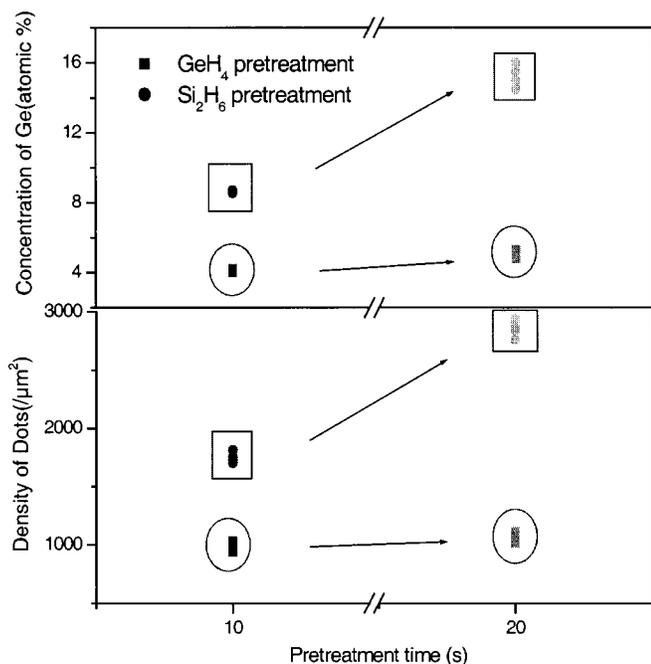
**Figure 6.** Comparison of Ge content in the SiGe dot vs. the density of dots after 10 and 20 s bursting of  $\text{Si}_2\text{H}_6$ , and  $\text{GeH}_4$ , respectively.
