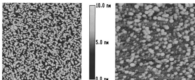
**Figure 5.** AFM image of the SiGe dots for 90 s with 0.75 gas ratio of  $\text{GeH}_4$  to  $\text{Si}_2\text{H}_6$  after the 20 s pretreatment step of different gases, (a)  $\text{Si}_2\text{H}_6$  or (b)  $\text{GeH}_4$  at  $525^\circ\text{C}$ , respectively.
