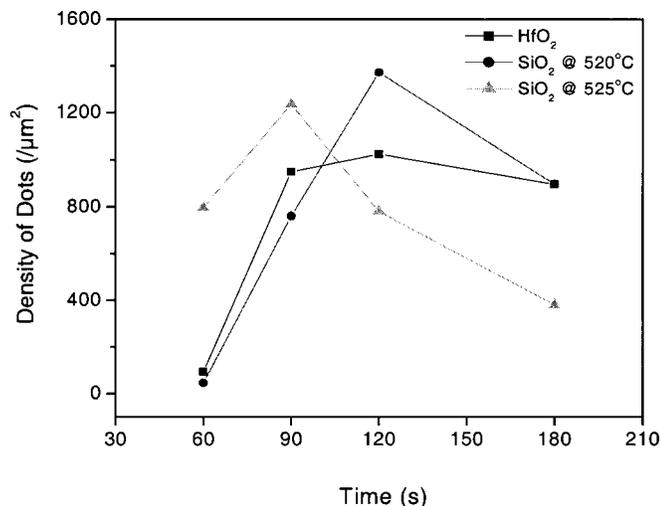
Figure 3. Dependence of density of dots on time and substrate temperature.
