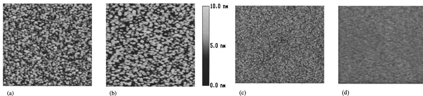
**Figure 1.** AFM scan images ( $1 \times 1 \mu\text{m}$ ) showing the self-assembled SiGe dots on (a)  $\text{HfO}_2$  and (b)  $\text{SiO}_2$  at 510 and 525°C respectively, for 90 s with 0.75 gas ratio of  $\text{GeH}_4$  to  $\text{Si}_2\text{H}_6$ . The vertical scale of the image is 10 nm, with white representing the highest point and black the lowest point in the images.
