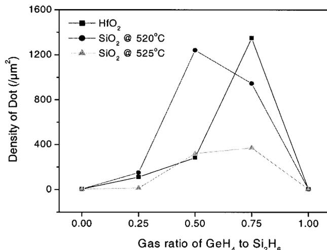
Figure 4. Summary of the SiGe dot density deposited on SiO<sub>2</sub> and HfO<sub>2</sub> substrates at the fixed temperatures vs. gas ratio of GeH<sub>4</sub> to Si<sub>2</sub>H<sub>6</sub>.
