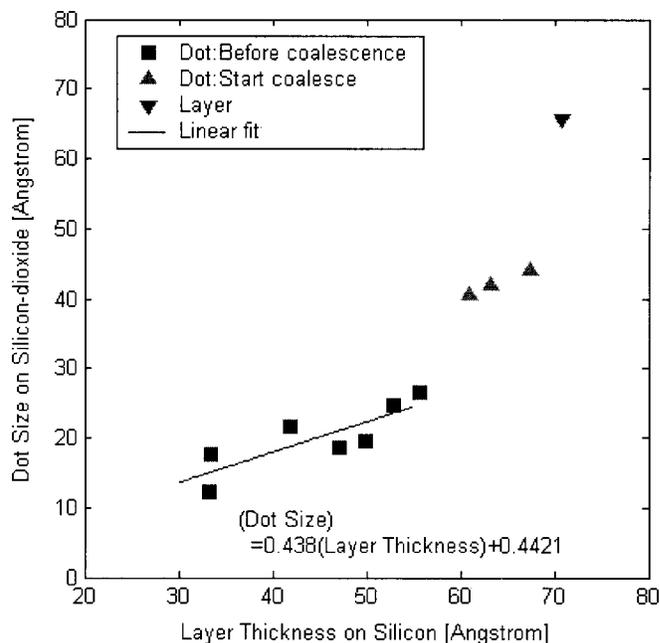
**Figure 7.** Relationship between dot size (before coalescence) formed on  $\text{SiO}_2$  and the thickness of layers on the Si substrate at the same process conditions in the temperature range of  $500\text{--}530^\circ\text{C}$ .
