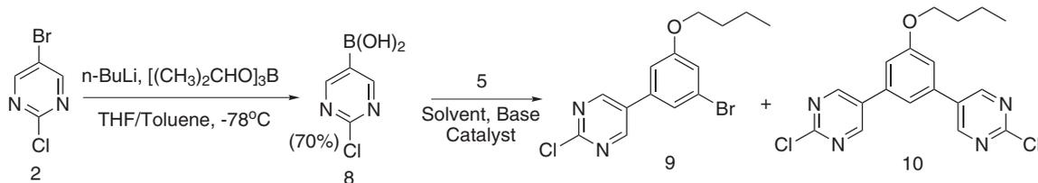
**Scheme 3.** Synthesis of dielectrophile with alkoxy side chain and reactive chloro substituents
