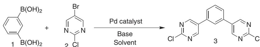
**Scheme 1.** Synthesis of dielectrophile from 1,3-phenylenebisboronic acid and 5-bromo-2-chloropyrimidine: (a) Pd(PPh<sub>3</sub>)<sub>4</sub>, Na<sub>2</sub>CO<sub>3</sub>, H<sub>2</sub>O, dioxane, reflux, 20 h; (b) Pd(PPh<sub>3</sub>)<sub>2</sub>Cl<sub>2</sub>, Na<sub>2</sub>CO<sub>3</sub>, dioxane, reflux, 25 h
