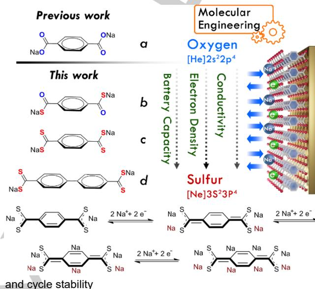
**Figure 1.** Schematic illustration of sulfur doping in molecular battery anode.
