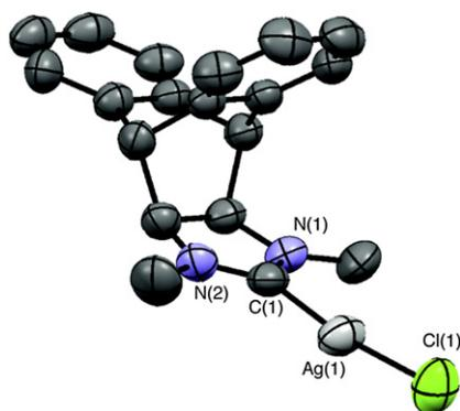
**Fig. 3.** ORTEP diagram of complex **16**, thermal ellipsoids are shown at 50% probability level. Selected bond length (Å) and angles (°): Cl(1)–Ag(1), 2.326; Ag(1)–C(1), 2.100; C(1)–N(1), 1.323; C(1)–N(2), 1.328; Cl(1)–Ag(1)–C(1), 171.64; Ag(1)–C(1)–N(1), 125.14; Ag(1)–C(1)–N(2), 126.00; N(1)–C(1)–N(2), 108.86.
