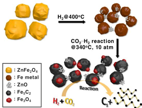
**Scheme 1.** Structural evolution and mechanistic idea of ZnFe<sub>2</sub>O<sub>4</sub>-derived catalyst for the selective synthesis of C<sub>5+</sub> liquid fuels by CO<sub>2</sub> hydrogenation.
