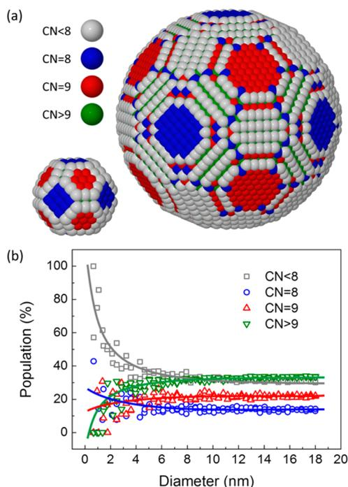
**Figure 5.** (a) Ball models of spherical Cu NPs with 2.2 and 6.9 nm diameters. Surface atoms are color-coded according to their first neighbor coordination number (CN), CN < 8 (gray), CN = 8 (blue), CN = 9 (red), CN > 9 (green). (b) Population (relative ratio) of surface atoms with a specific CN as a function of particle diameter.
