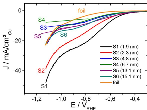
**Figure 2.** Linear sweep voltammetry of the CO<sub>2</sub> electroreduction on Cu NP catalysts, S1–S6, in 0.1 M KHCO<sub>3</sub> acquired at room temperature with  $-5$  mV/s scan rate. Current densities are normalized by the Cu particle surface area after subtraction of the glassy carbon background signal. A Cu foil electrode (“foil”) is included as reference.
