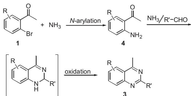
**Scheme 1.** Proposed mechanism for CuCl-catalyzed formation of quinazolines.
