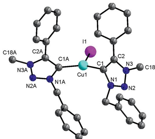
Figure 1. ORTEP plot of  $6 \cdot \text{CH}_2\text{Cl}_2$ . Ellipsoids are drawn at 50% probability. Hydrogen atoms and solvent molecules have been omitted for clarity.
