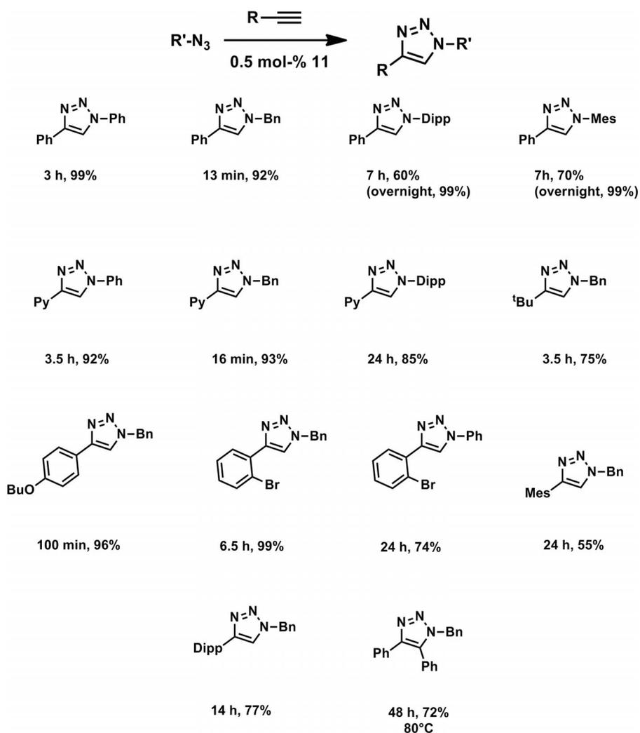
Scheme 4. The range of substrates tested with catalyst **11**.
