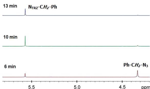
Figure 4. <sup>1</sup>H NMR spectra of the benzylic CH<sub>2</sub> protons of reactant and product showing the completion of the reaction shown in Scheme 5.
