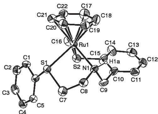
**Figure 3.** ORTEP diagram of cation of **4** with 30% probability ellipsoids. Hydrogen atoms (except NH), H<sub>2</sub>O, Cl, and PF<sub>6</sub> are omitted for clarity. Bond lengths (Å): Ru(1)–S(1) 2.374(3), Ru(1)–S(2) 2.379(2), Ru(1)–N(1) 2.135(5), Ru(1)–C 2.146(15)–2.218(9). Bond angles (deg): S(1)–Ru(1)–S(2) 90.75(10), N(1)–Ru(1)–S(1) 83.0(2), N(1)–Ru(1)–S(2) 86.51(18).
