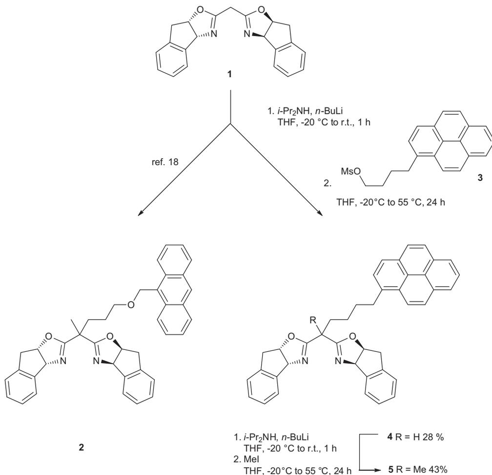
**Scheme 1.** Synthetic procedure for the synthesis of bis(oxazoline) ligands **2** and **5**.
