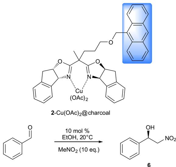
**Scheme 2.** Nitroaldol reaction in the presence of **2-Cu(OAc)<sub>2</sub>@charcoal**.
