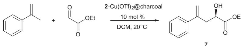
**Scheme 3.** Ene reaction between ethyl glyoxylate and  $\alpha$ -methylstyrene in the presence of **2**-Cu(OTf)<sub>2</sub>@charcoal.
