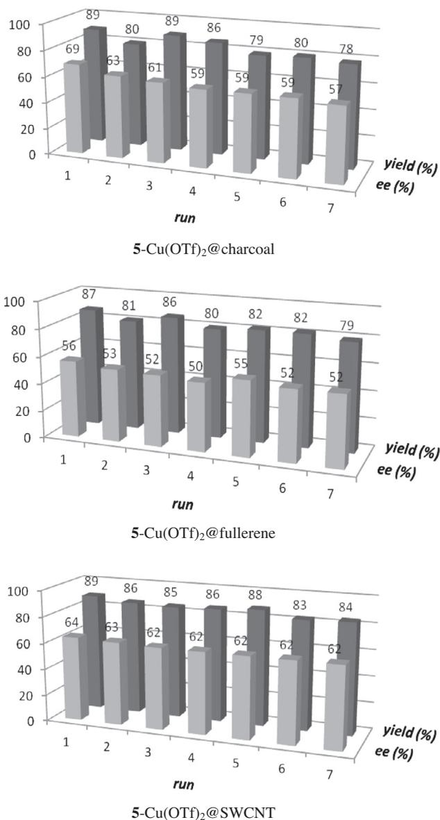
**Figure 3.** The ene reaction between ethyl glyoxylate and  $\alpha$ -methylstyrene at 20 °C for 16 h in the presence of the supported catalysts (10 mol %) [formation of (*R*)-**7** as the main product].
