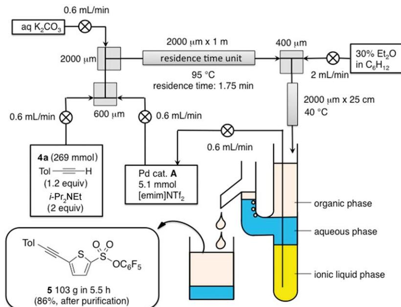
**Scheme 8** Synthesis of **5** on a 100 gram scale using a continuous-flow and catalyst-/solvent-recycling system
