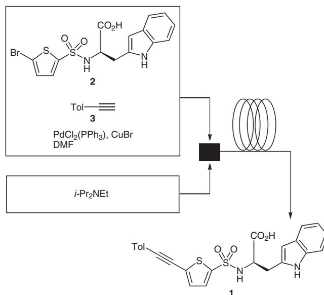
**Scheme 1** Microflow synthesis of MMP inhibitor **1**<sup>5</sup>
