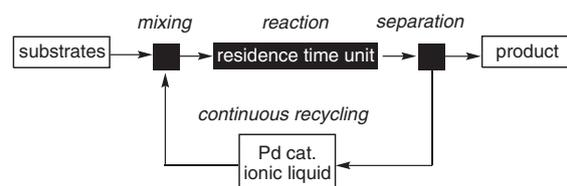
**Scheme 2** Concept of a continuous catalyst-recycling system using an IL as a reaction medium
