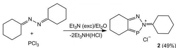
**Scheme 2.** Reaction of *c*-HA with  $\text{PCl}_3$  in diethyl ether. Formation of 2-cyclohexylidene-4,5,6,7-tetrahydro-2H-1,2,3-benzodiazaphospholium chloride (**2**).
