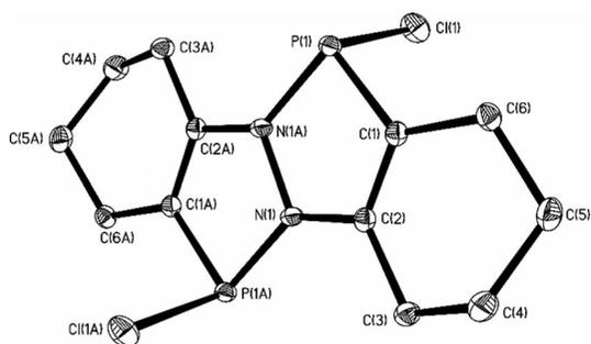
**Figure 1.** The molecular structure of **1** with ellipsoids of 30% probability. Hydrogen atoms are omitted for clarity. Selected bond lengths /Å and angles /° for **1**: P(1)–N(1A) 1.693(1), P(1)–C(1) 1.798(2), P(1)–Cl(1) 2.1762(6), N(1)–C(2) 1.390(2), N(1)–N(1A) 1.413(2), C(1)–C(2) 1.347(2); N(1A)–P(1)–C(1) 88.11(6), N(1A)–P(1)–Cl(1) 104.35(5), C(1)–P(1)–Cl(1) 99.09(5), C(2)–N(1)–N(1A) 109.5(1). Symmetry transformations used to generate equivalent atoms A:  $-x, -y, -z$ .
