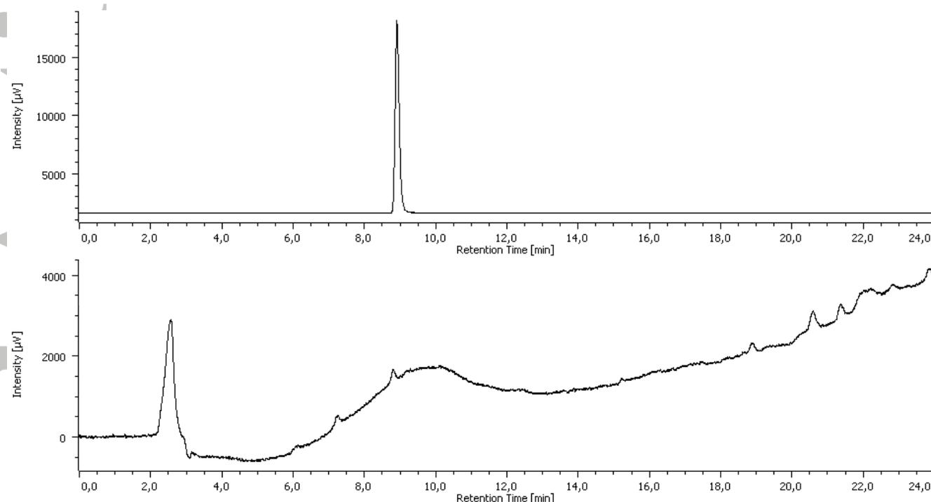
**Figure 4 – RP-HPLC profile of purified product [ $^{18}\text{F}$ ]**18** by semipreparative RP-HPLC. [ $^{18}\text{F}$ ]**18** retention time was 8.9 min (water/acetonitrile gradient from 90:10 to 30:70 in 24 min, 1 ml/min flow, 220 nm/radiochemical detector).**
