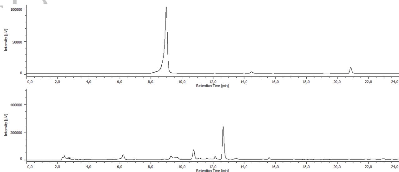
**Figure 3** – RP-HPLC profile of pre-purified product [<sup>18</sup>F]18 from catalyst system. [<sup>18</sup>F]18 retention time was 8.9 min, [<sup>18</sup>F]1 retention time was 20.9 min. (water/acetonitrile gradient from 90:10 to 30:70 in 24 min, 1 ml/min flow, 220 nm/radiochemical detector).
