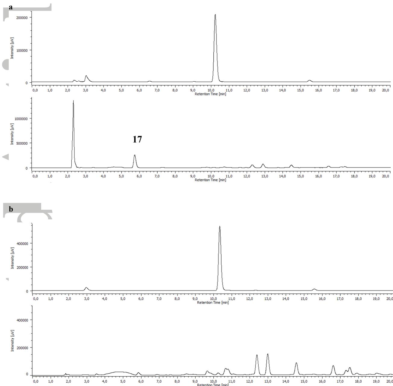
**Figure 2** – RP-HPLC profile of crude (a) and purified [ $^{18}\text{F}$ ]**1** (b), obtained from precursor **4**. [ $^{18}\text{F}$ ]**1** retention time was 10.2 min (water/acetonitrile gradient from 60:40 to 20:80 in 20 min, 1 ml/min flow, 220 nm/radiochemical detector).
