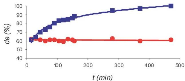
Figure 4 Conjugate addition of (*R,R*)-**1** to  $\alpha,\beta$ -unsaturated malonate **7d** using  $\text{Fe}_2\text{O}_3\text{-KOH}$  as base in anhydrous (red circles) or wet (blue squares)  $\text{CH}_2\text{Cl}_2$
