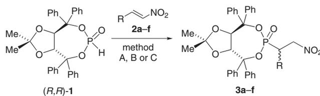
**Scheme 1** Reagents and conditions: Method A: *n*-BuLi, THF, 0 °C, 40 h. Method B: Et<sub>2</sub>Zn, THF, –78 °C to r.t., 12 h. Method C: Et<sub>2</sub>Zn, TMEDA, THF, –78 °C, 12 h.
