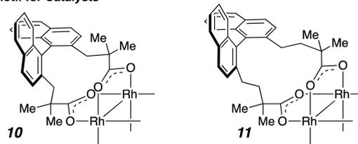
**Figure 1.** Rhodium(II) complexes with biscarboxylate ligands. Undefined ligands are identical to the one illustrated to provide a symmetric complex, with the exception of complexes **2d** and **2e**, which have two different R<sup>3</sup> groups.
