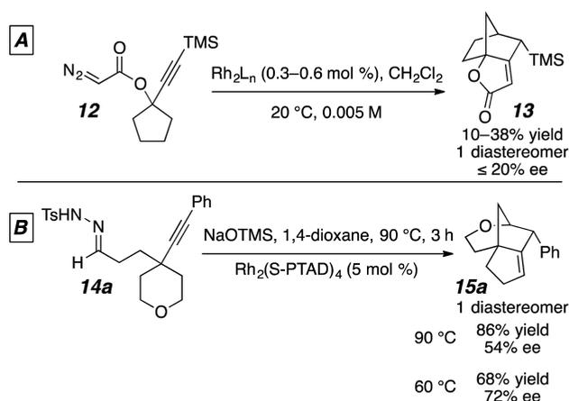
Figure 3. Use of known chiral catalysts in the carbene/alkyne cascade.<sup>12</sup>
