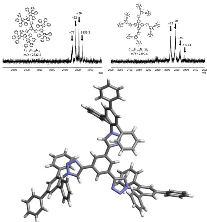
**Fig. 4.** MALDI-TOF of polyphenylene-triazole compounds **13** (up left) and **16** (up right). Single crystal structure of first generation polyphenylene-triazole dendrimer **9** with a trigonal planar core (mid). For crystallographic data of compound **9** see [Supplementary data](#) and the Cambridge Crystallographic Data Centre (CCDC).
