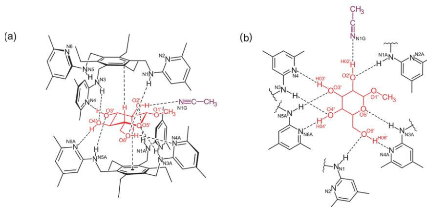
Figure 10. Schematic representation of the pattern of hydrogen bonds (shown as dashed lines) formed between the receptor **3** and methyl  $\beta$ -D-glucopyranoside in complex I [(**3**)<sub>2</sub>-**MeβGlc-I**]. The carbohydrate molecule is displayed in red, the solvent molecule in violet. Only one disordered position of the solvent molecule is shown.
