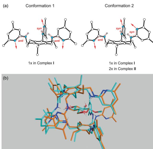
Figure 11. (a) Conformations of the receptor molecules in the crystal structure **3·Me $\beta$ Glc**. (b) A view of superposition of **(3)<sub>2</sub>·Me $\beta$ Glc-I** (orange lines) and **(3)<sub>2</sub>·Me $\beta$ Glc-II** (light blue lines) fitting on the carbohydrate atoms C1–C5 and O5 (N atoms are colored blue and O atoms red; all non-polar hydrogens omitted for clarity).
