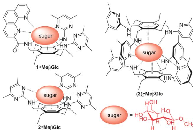
Figure 1. Schematic illustration of the 1:1 and 2:1 receptor-sugar complexes, the crystal structures of which are discussed in this paper.
