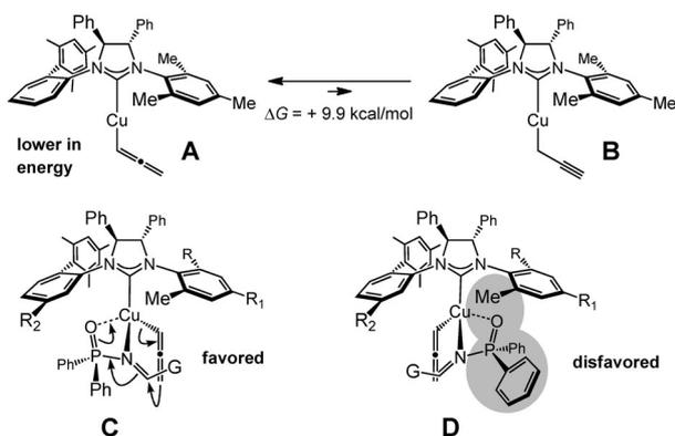
**Scheme 5.** Theoretical studies point to a strong energetic preference for the NHC–Cu–allenyl **A** versus the derived propargyl complex **B** and a model that accounts for the observed stereochemical outcomes.
