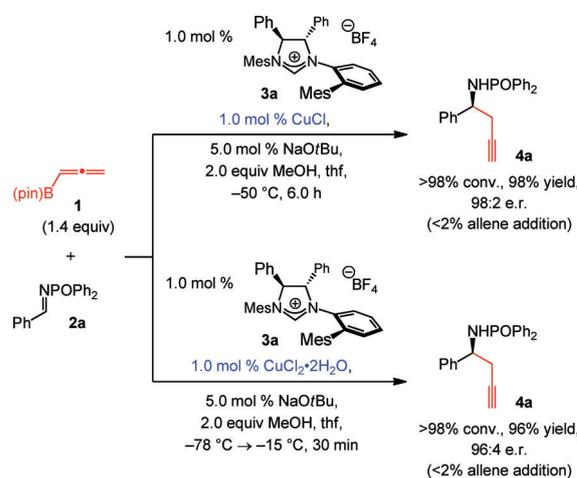
**Scheme 2.** NHC–Cu-catalyzed propargyl addition can be performed with CuCl or the air-stable CuCl<sub>2</sub>·2H<sub>2</sub>O with exceptional efficiency and high enantioselectivity. Mes = 2,4,6-(Me)<sub>3</sub>C<sub>6</sub>H<sub>2</sub>.
