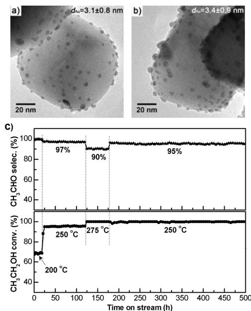
**Figure 1.** TEM images of a) fresh Au/MgCuCr<sub>2</sub>O<sub>4</sub> catalyst, b) used Au/MgCuCr<sub>2</sub>O<sub>4</sub> catalyst after 500 h on-stream; c) ethanol conversion and acetaldehyde selectivity vs time on stream using Au/MgCuCr<sub>2</sub>O<sub>4</sub> (Reaction conditions: catalyst 0.1 g, GHSV = 100,000 mL g<sub>cat</sub><sup>-1</sup> h<sup>-1</sup>, ethanol/O<sub>2</sub>/He = 1/3/63).
