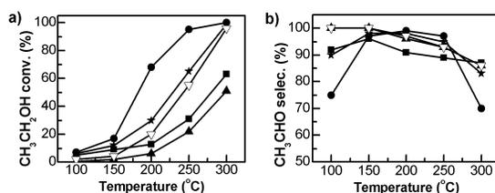
**Figure 2.** Temperature-dependent ethanol oxidation over various catalysts showing a) ethanol conversion, b) acetaldehyde selectivity. (●) Au/MgCuCr<sub>2</sub>O<sub>4</sub>, (★) Au/MgCuAl<sub>2</sub>O<sub>4</sub>, (■) Au/TiO<sub>2</sub>, (▲) Au/MgCr<sub>2</sub>O<sub>4</sub> and (▽) Au/CuO-SiO<sub>2</sub>.
