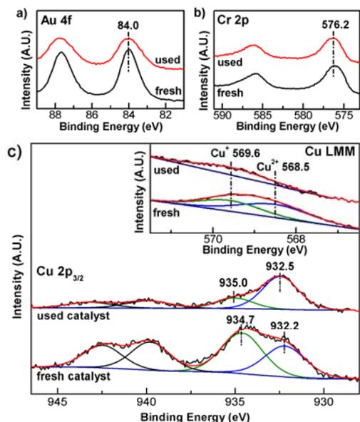
**Figure 3.** XP spectra of the Au/MgCuCr<sub>2</sub>O<sub>4</sub> catalyst before and after 500 h on stream. a) Au 4f XP spectra, b) Cr 2p XP spectra, c) Cu 2p<sub>3/2</sub> and Cu LMM (inset) XP spectra.
