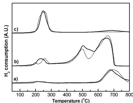
**Figure 4.** H<sub>2</sub> consumption traces (TPR) of a) Au/MgCuCr<sub>2</sub>O<sub>4</sub>, b) Au/CuCr<sub>2</sub>O<sub>4</sub>, and c) Au/MgCuAl<sub>2</sub>O<sub>4</sub> catalysts. The dashed line represents the trace of the corresponding spinel support.
