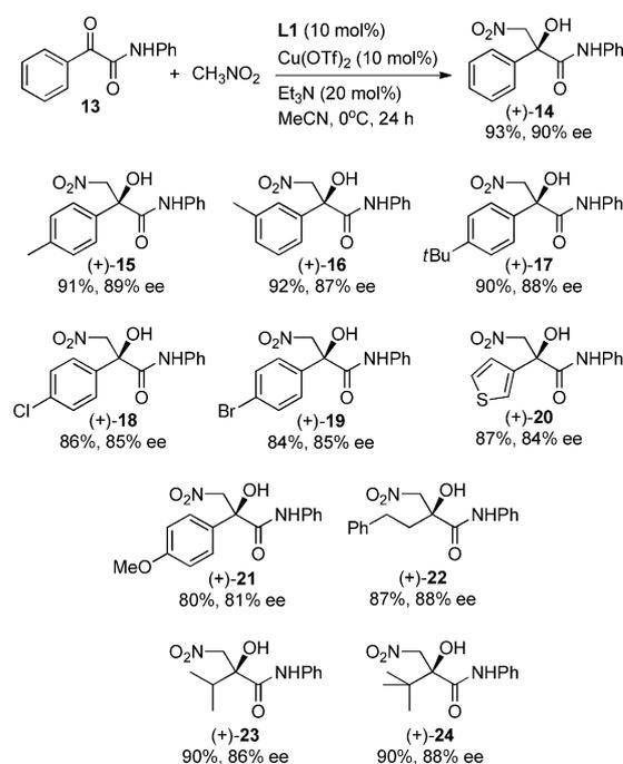
**Scheme 4.** Enantioselective synthesis of 2-substituted 2-hydroxy-3-nitropropanamides by using 10 mol % of  $\text{Cu}(\text{OTf})_2$  and ligand **L1**. Tf = trifluoromethanesulfonyl.
