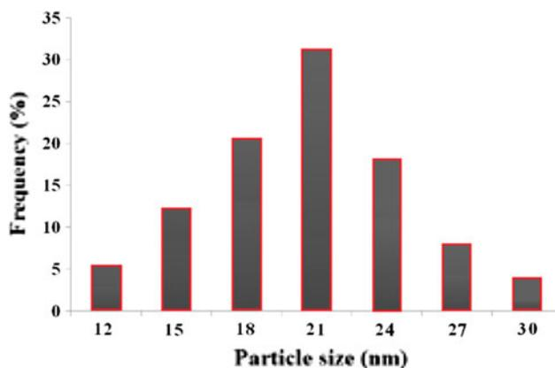
**Fig. 2** Histogram representing the size distribution of Pd nanoparticles on SBPPSP substrate
