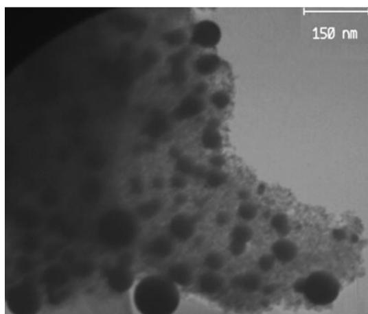
**Fig. 1** Transmission electron microscope (TEM), which show the image of Pd nanoparticle on SBPPSP support
