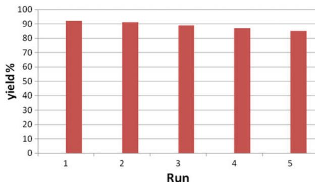
**Fig. 5** Recyclability of PNP-SBPPSP in the reaction of iodobenzene (2 mmol), phenylacetylene (2.4 mmol), triethylamine (8 mmol) and acetonitrile (5 mL) under reflux conditions. Reaction time = 1.0 h
