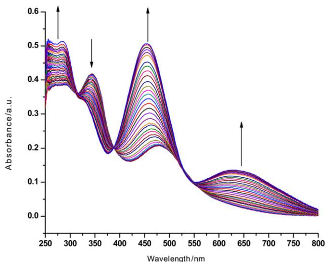
Fig. 6. UV-vis spectral titration of sensor CS3 with Cu<sup>2+</sup> in DMSO solution.
