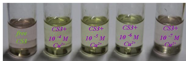
Fig. 9. Color changes observed upon the addition of varying quantities of  $\text{Cu}^{2+}$  (from left to right: free **CS3**,  $1 \times 10^{-4}$  M,  $1 \times 10^{-5}$  M,  $1 \times 10^{-6}$  M,  $1 \times 10^{-7}$  M) to the solutions of sensor **CS3** ( $1 \times 10^{-5}$  M; DMSO/ $\text{H}_2\text{O}$ , 9:1, v:v; HEPES buffered, pH 7.0). (For interpretation of the references to color in this figure legend, the reader is referred to the web version of this article.)
