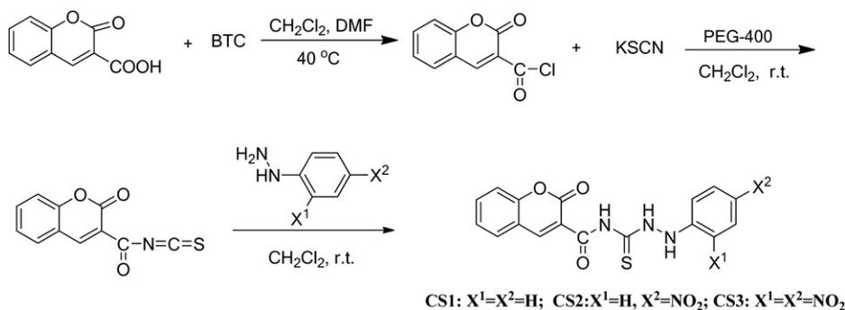
**Scheme 1.** Synthetic procedures for sensors **CS1**–**CS3**.
