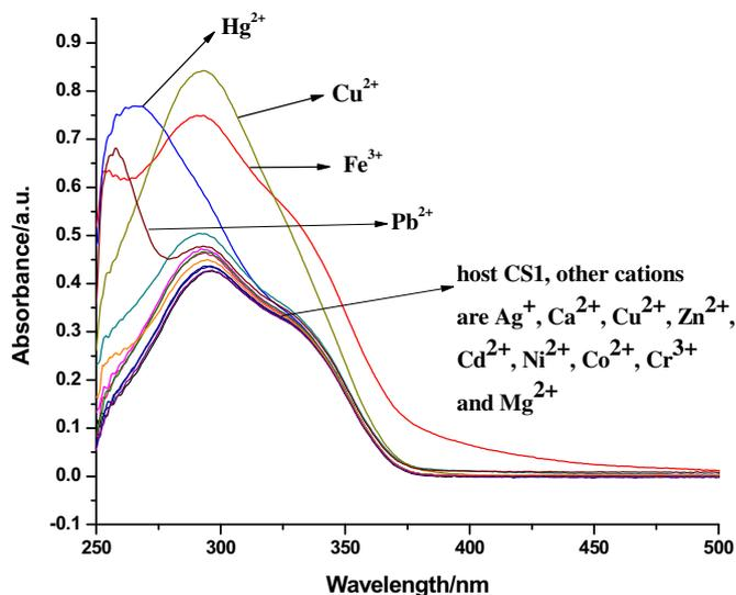
Fig. 4. UV-vis absorption spectra of CS1 in the presence of 5 equiv. of various cations in DMSO/H<sub>2</sub>O (9:1, v/v; HEPES buffered, pH 7.0) solution at room temperature.
