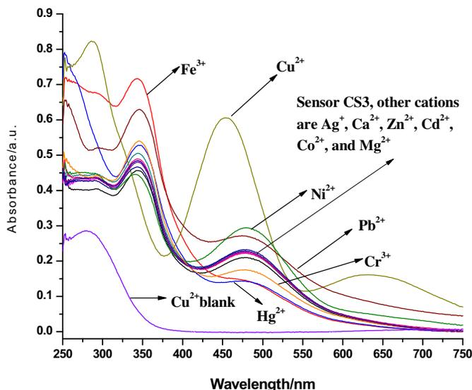
Fig. 2. UV-vis absorption spectra of CS3 in the presence of 5 equiv. of various cations in DMSO/H<sub>2</sub>O (9:1, v/v; HEPES buffered, pH 7.0) solution at room temperature.
