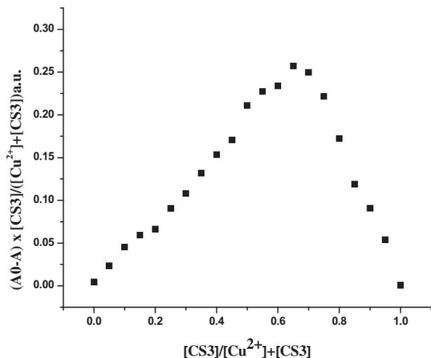
Fig. 5. (a) A Job plot of CS3 and Cu<sup>2+</sup>, which indicated that the stoichiometry of CS3-Cu<sup>2+</sup> complex was 2:1.
