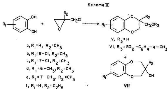
reaction mixture as tosylates VI (Table IV) (7), from which then they were easily obtained in pure state by alkaline hydrolysis. Carbinols VII, being more resistant than V to oxidation, were easily recovered from the potassium permanganate oxidation mixture, simply by extracting the final alkaline solution with ether. The dioxepines VIId and VIIf could also be isolated as unreacted material during the preparation of the tosylates of the corresponding benzodioxane alcohols (see Experimental).
