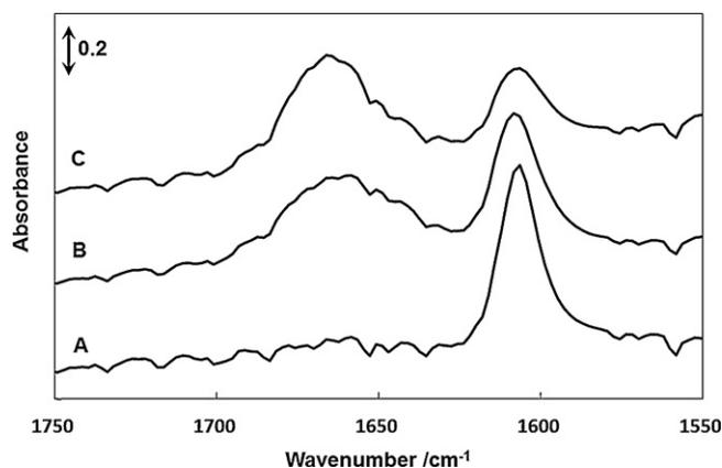
**Fig. 11.** IR spectra of surface species remaining on (A) Cs-X, (B) ZrB/Cs-X and (C) ZnB/Cs-X after exposure to 133 Pa methanol at 623 K followed by cooling down to room temperature.
