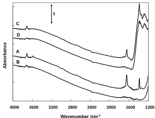
Fig. 9. IR spectra of CO<sub>2</sub> adsorbed on Cs-X and ZrB/Cs-X. (A and B) CO<sub>2</sub> adsorbed on Cs-X and evacuated at 373 K and 523 K, respectively; (C and D) CO<sub>2</sub> adsorbed on ZrB/Cs-X and evacuated at 373 K and 523 K, respectively.
