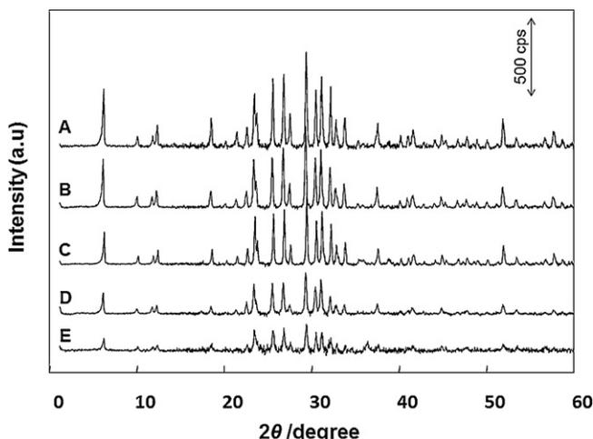
**Fig. 5.** XRD patterns of Cs-X and Cs-X's modified with metal borates. (A) Cs-X, (B) ZrB/Cs-X, (C) CuB/Cs-X, (D) LaB/Cs-X and (E) ZnB/Cs-X.
