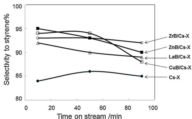
Fig. 2. Selectivity to styrene as a function of time on stream in side chain alkylation of toluene with methanol at 683 K over Cs-X and Cs-X's modified with metal borates.
