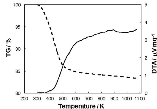
Fig. 8. TG/DTA of ZrB/Cs-X. Dotted line, TG; solid line, DTA.
