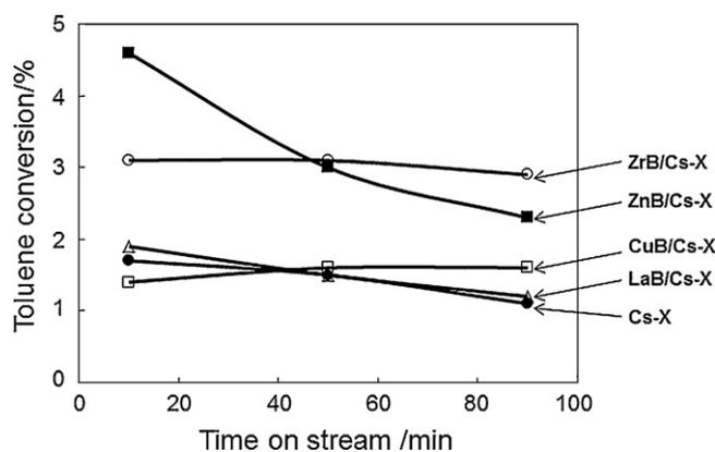
Fig. 1. Toluene conversion as a function of time on stream in side chain alkylation of toluene with methanol at 683 K over Cs-X and Cs-X's modified with metal borates.
