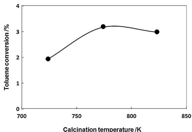
Fig. 4. Variation in toluene conversion as a function of calcination temperature of ZrB/Cs-X in side chain alkylation of toluene with methanol at 683 K.
