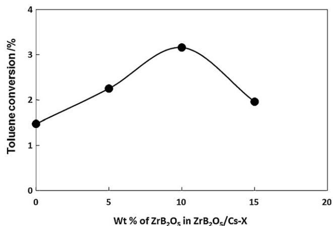
Fig. 3. Variation in toluene conversion as a function of zirconium borate loading of ZrB/Cs-X in side chain alkylation of toluene with methanol at 683 K.
