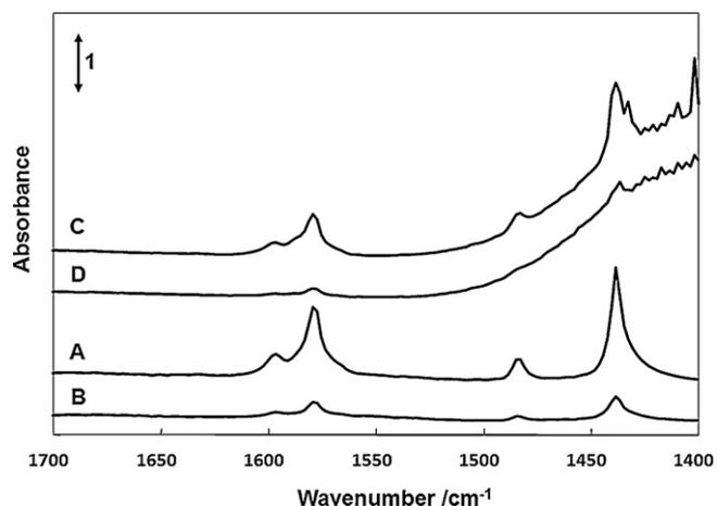
Fig. 10. IR spectra of pyridine adsorbed on Cs-X and ZrB/Cs-X. (A and B) Pyridine adsorbed on Cs-X and evacuated at 473 K and 523 K, respectively; (C and D) pyridine adsorbed on ZrB/Cs-X and evacuated at 473 K and 523 K, respectively.
