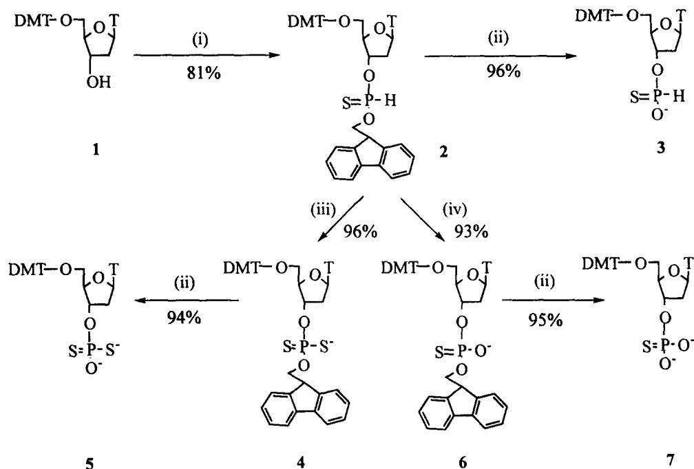
**Figure 1.** Synthesis of nucleotide analogs via a common intermediate. (i) tris-pyrrolidinylphosphine, 9-fluorenylmethanol, H<sub>2</sub>S, 1-H-tetrazole; (ii) 20% piperidine/CH<sub>2</sub>Cl<sub>2</sub>; (iii) Sg/CS<sub>2</sub>/pyridine; (iv) 0.1 M I<sub>2</sub> in THF/pyridine/H<sub>2</sub>O (2/2/1).
