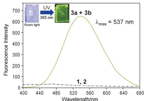
**Fig. 6** Solid-state photoluminescence spectra of **1**, **2** and **3a** (with small amount of **3b**) at room temperature (excitation at 343 nm).
