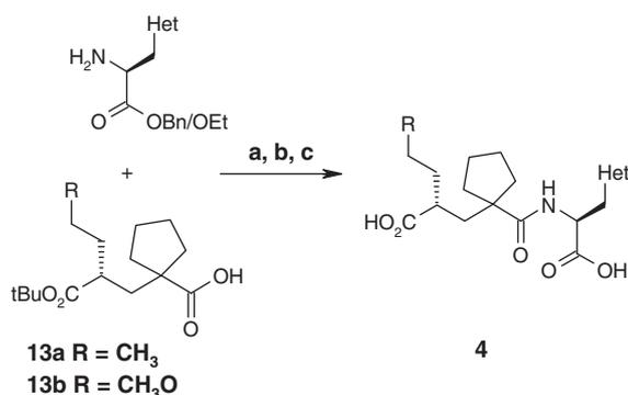
**Scheme 3.** Reagents and conditions: (a) WSCDI, HOBT, NMM, DCM, 50–92%; (b) TFA, DCM, 85–98%; (c) NaOH, dioxan,  $\text{H}_2\text{O}$ , 53–96%.
