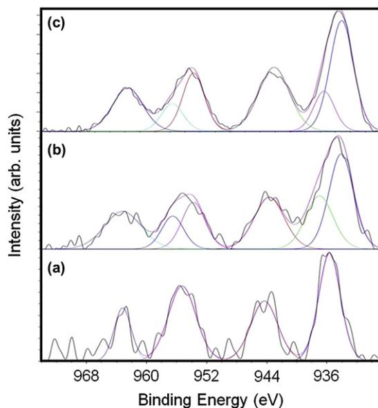
Fig. 2. High resolution narrow X-ray photoelectron spectra (XPS) for (a) fresh clay supported Cu(II) catalyst; (b) clay–Cu(II) catalyst treated with sodium azide; (c) CuSO<sub>4</sub> treated with NaN<sub>3</sub>.
