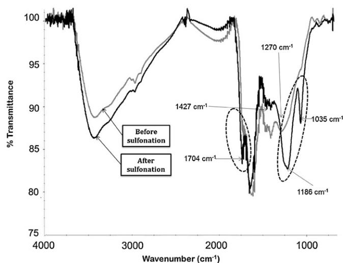
**Fig. 3.** FTIR spectra of the TAC-673 materials prepared from sucrose before and after sulfonation.
