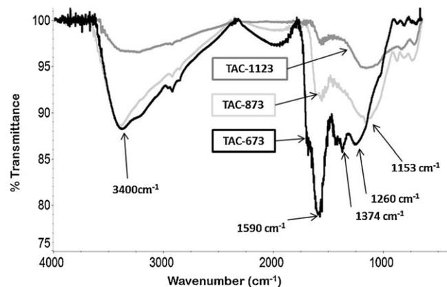
**Fig. 2.** Infrared spectra of the TAC carbonized materials at different temperatures.
