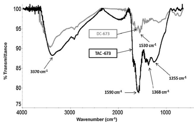
**Fig. 1.** Infrared spectra of the carbonized materials. Top: DC carbonized material at 673 K. Bottom: TAC carbonized material at 673 K.
