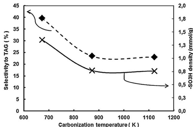
Fig. 4. Selectivity to TAG by esterification of glycerol with acetic acid (9:1 molar relation, at 433 K and 5% of catalyst load). (Black rhombus) effect of the temperature of carbonization of the catalysts. (Equis) effect of SO<sub>3</sub>H density sites. The connecting lines in figure are just a guide for the eyes.
