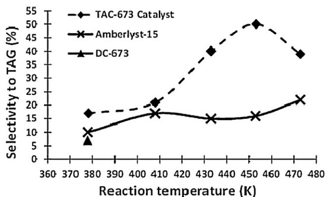
Fig. 5. Selectivity to TAG by esterification of glycerol with acetic acid (at 9:1 molar relation, 5% of catalyst load and 4 h of reaction time). Black rhombus for TAC-673. Equis for commercial catalyst (Amberlyst-15). Black triangle for DC-673 catalyst. The connecting lines in figure are just a guide for the eyes.
