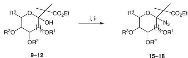
**Scheme 3** Reagents and conditions: (i)  $\text{Ac}_2\text{O}$ ,  $\text{Et}_3\text{N}$ ,  $\text{CH}_2\text{Cl}_2$ , r.t., 14 h; (ii)  $\text{TMSN}_3$ ,  $\text{TMSOTf}$ , powdered MS,  $\text{CH}_2\text{Cl}_2$ , r.t., 14 h.
