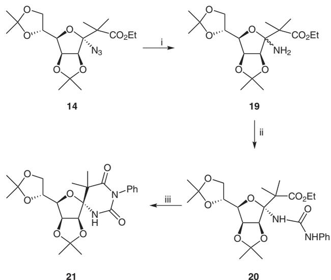
**Scheme 4** Reagents and conditions: (i) Pd/C, MeOH, r.t., 14 h; (ii) PhCON, toluene, r.t., 3 h; (iii) NaOMe, r.t., 14 h.
