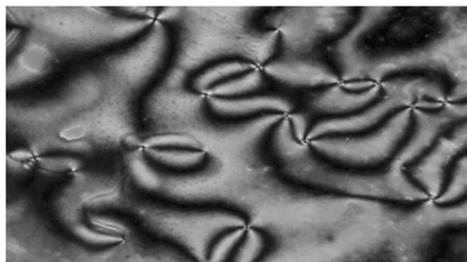
Compound **1c**,  $137^\circ\text{C}$ , fourth cooling**FIGURE 7** Photomicrograph of some ferrocene containing liquid crystals.
