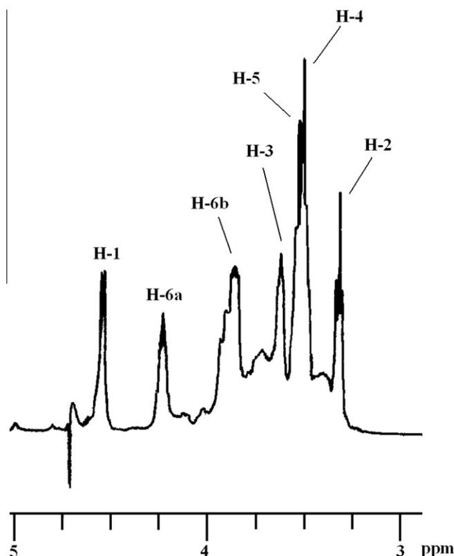
**Figure 1.** <sup>1</sup>H NMR spectrum (500 MHz, D<sub>2</sub>O, 27 °C) of PS-I, isolated from fruit bodies of hybrid mushroom.
