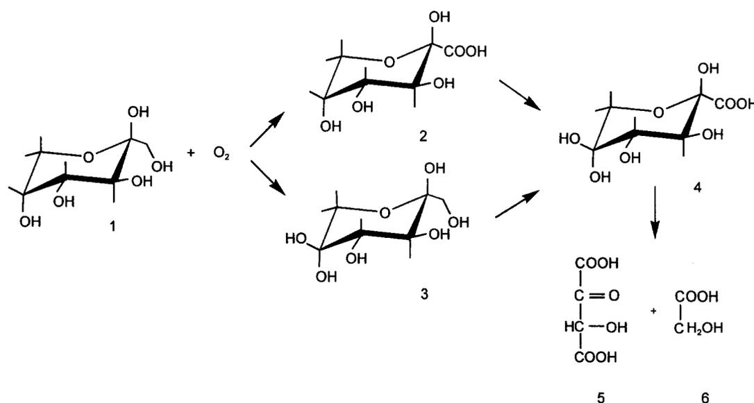
Scheme 2. Oxidation products of fructose (1), 2-ketogluconic acid (2), *D-threo*-hexo-2,5-diulose (3), 2,5-diketogluconic acid (4), 2-hydroxy-3-butanedioic acid (5) and glycolic acid (6).
