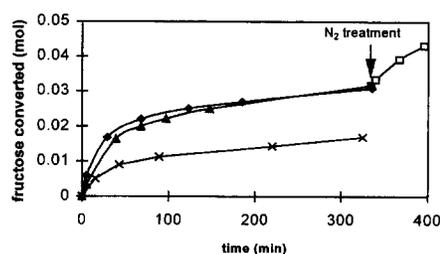
Fig. 2. Oxidation of fructose on Pt/C (batch 3).  $T$  30 °C, pH 7.3,  $pO_2$  0.2 atm, [fructose] = 12.5 g/L, [5 wt.% Pt/C] = 6.3 g/L. Fructose converted on fresh (◆) and used catalyst before (▲) and after nitrogen treatment (□) and with 3.1 g/L 2-ketogluconic acid in the initial reaction mixture (x).
