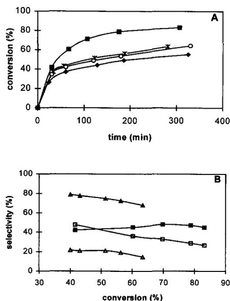
Fig. 3. Oxidation of fructose on different BiPt/C catalysts. *T* 30 °C, pH 7.3, pO<sub>2</sub> 0.2 atm, [fructose] = 12.5 g/L, [5 wt.% Pt/C] = 6.3 g/L. (A) Conversion of fructose versus reaction time on ■, Pt/C; \*, BiPt/C (precipitation); ○, BiPt/C (glucose); ◆, BiPt/C (hydrogen). (B) Selectivity to 2-ketogluconic acid (closed figures) and '5-ketofructose' (open figures) versus fructose conversion: △/▲, BiPt/C (precipitation); □/■, Pt/C.
