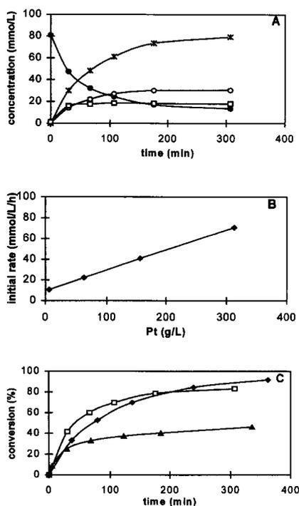
Fig. 1. Oxidation of fructose.  $T$  30 °C, pH 7.3,  $pO_2$  0.2 atm, [fructose] = 12.5 g/L, [5 wt.% Pt/C] = 6.3 g/L. (A) Concentrations of fructose (●), 2-ketogluconic acid (○), '5-ketofructose' (□) and the amount NaOH added (\*) versus reaction time (catalyst: Pt/C batch 2). (B) Initial rate versus catalyst concentration. (C) Conversion of fructose on different batches 5 wt.% Pt/C; ◆, batch 1; □, batch 2; ▲, batch 3.
