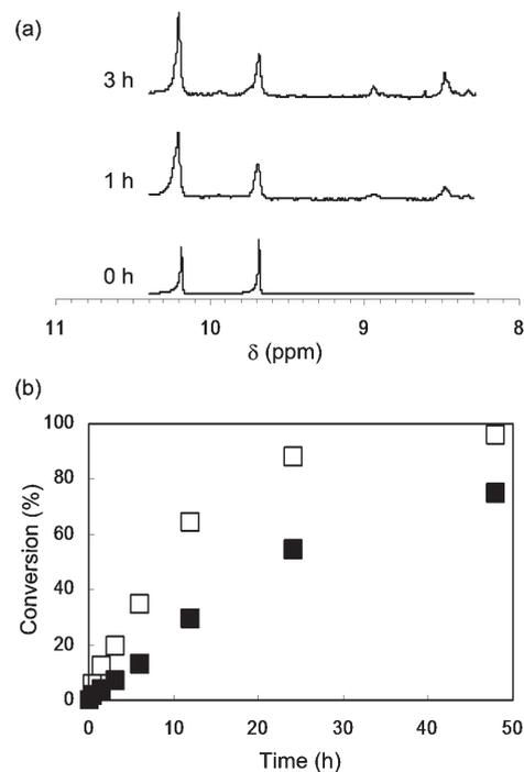
**Figure 2.** (a) Typical <sup>1</sup>H NMR spectra at the initial stage of the AB-type aza-Wittig polymerization and (b) consumption rate of **M1b** (open squares) and **M2b** (filled squares).
