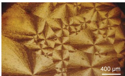
Fig. 9 Microphotograph of  $[\text{PdCl}_2(\text{Hpz}^{\text{R}(14,14)\text{py}})]$  **22** at 153 °C on cooling (type II).
