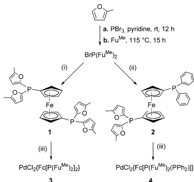
**Scheme 1.** Reagents and conditions: (i) 0.5 equivs.  $\text{FeCp}_2\text{Li}_2$ -TMEDA, hexane, room temperature, 2 h; (ii) 1 equiv.  $\text{CpFe}\{\text{Cp}(\text{PPh}_2)\}\text{Li}$ , THF,  $-50^\circ\text{C}$ , 12 h; (iii) 1 equiv.  $\text{PdCl}_2(\text{PhCN})_2$ ,  $\text{CH}_2\text{Cl}_2$ , room temperature, 20 min.
