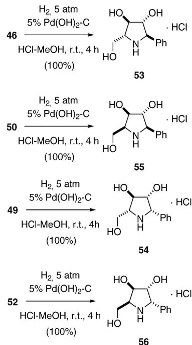
Scheme 11. Synthesis of 2-phenyl-substituted polyhydroxylated pyrrolidines.
