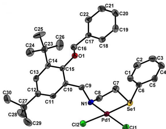
**Fig. 2** ORTEP representation of **2**. Selected bond lengths (Å) and angles (°): Pd1–N1 2.066(3), Pd1–Se1 2.366(1), Pd1–Cl1 2.306(1), Pd1–Cl2 2.331(1); N1–Pd1–Cl1 176.0(1), N1–Pd1–Cl2 88.0(1), Cl1–Pd1–Cl2 95.1(1), N1–Pd1–Se1 88.9(2), Cl1–Pd1–Se1 87.9(4), Cl2–Pd1–Se1 176.8(1).
