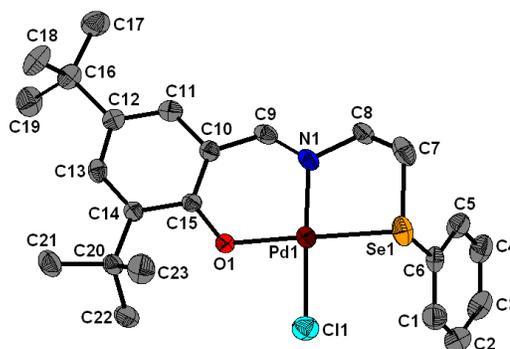
Fig. 1 ORTEP representation of **1**. Selected bond lengths (Å) and angles (°): Pd1–N1 1.996(4), Pd1–O1 2.001(3), Pd1–Se1 2.370(1), Pd1–Cl1 2.302(1); N1–Pd1–O1 92.5(2), N1–Pd1–Cl1 178.3(1), O1–Pd1–Cl1 88.3(1), N1–Pd1–Se1 89.1(1), O1–Pd1–Se1 177.2(1), Cl1–Pd1–Se1 90.1(1).
