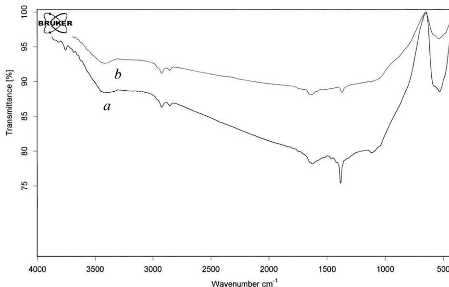
Fig. 1. IR spectra of CuO: (a) newly prepared; (b) used 3 times.
