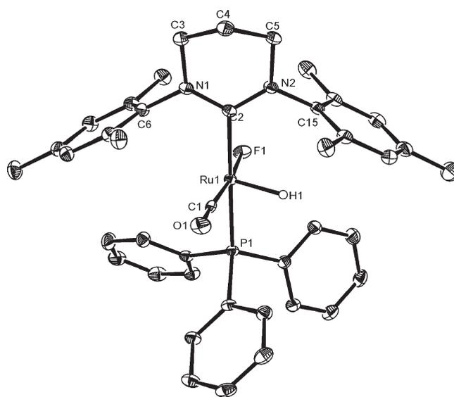
**Figure 1.** X-ray crystal structure of Ru(6-Mes)(PPh<sub>3</sub>)(CO)HF (**1**). Thermal ellipsoids are set at 30% probability. Hydrogen atoms (except Ru–H) and minor disordered components have been omitted for clarity. Selected bond lengths (Å) and angles (deg): Ru(1)–C(1) 1.821(7), Ru(1)–C(2) 2.1041(18), Ru(1)–P(1) 2.3294(5), Ru(1)–F(1) 2.0418(11), C(2)–Ru(1)–P(1) 177.82(5), C(1)–Ru(1)–F(1) 172.92(13), N(1)–C(2)–N(2) 117.17(16).
