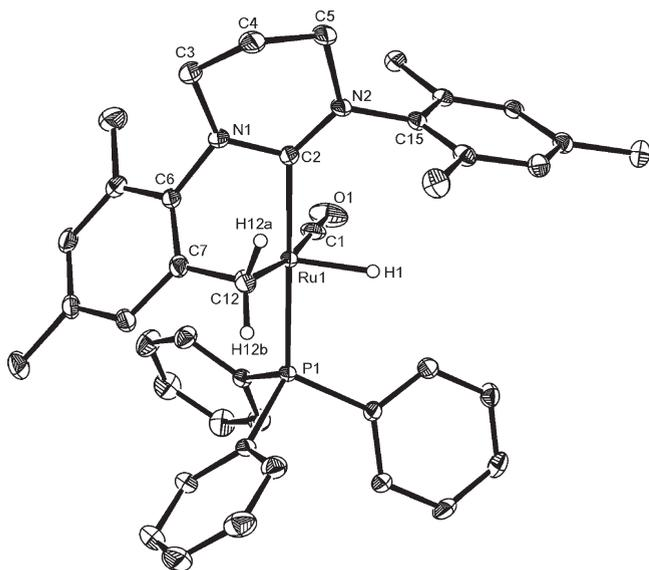
**Figure 2.** X-ray crystal structure of Ru(6-Mes)(PPh<sub>3</sub>)(CO)H (**2**). Thermal ellipsoids are set at 30% probability. Hydrogen atoms (except for Ru–H and Ru–CH<sub>2</sub>) have been omitted for clarity, as have the solvent and the minor disordered components present. Selected bond lengths (Å) and angles (deg): Ru(1)–C(1) 1.847(3), Ru(1)–C(2) 2.063(2), Ru(1)–C(12) 2.228(2), Ru(1)–P(1) 2.3339(6), C(2)–Ru(1)–P(1) 178.11(7), C(1)–Ru(1)–C(12) 171.45(10), N(1)–C(2)–N(2) 118.7(2).
