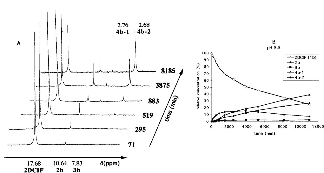
**Figure 3.** Stack plot of <sup>31</sup>P NMR spectra recorded during 2DCIF (**1b**) hydrolysis in 0.1 M cacodylate buffer at pH 5.5, 25 °C (A). Corresponding <sup>31</sup>P NMR time course (B).
