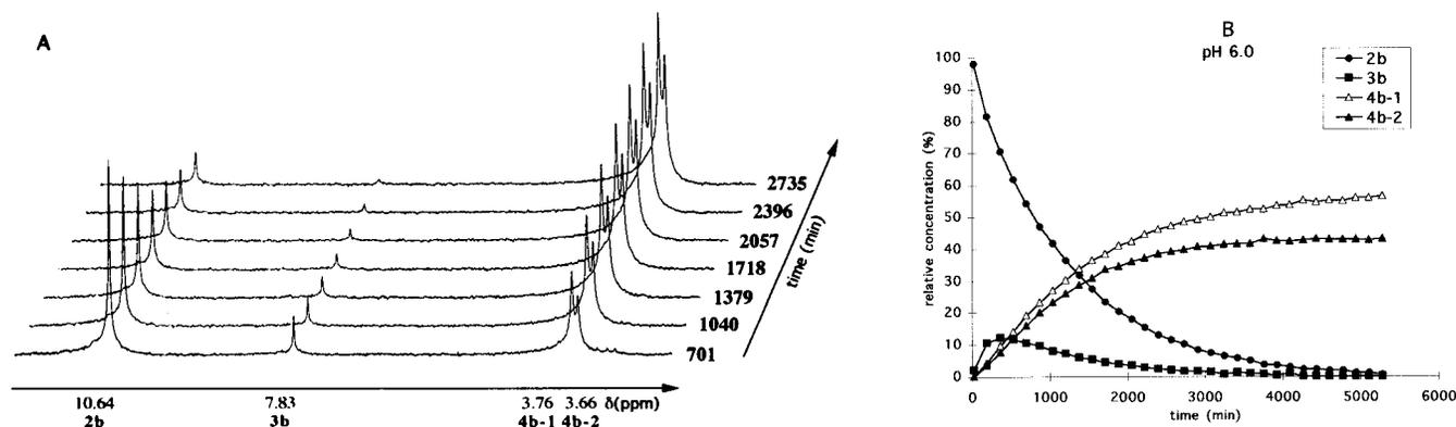
**Figure 5.** Stack plot of  $^{31}\text{P}$  NMR spectra recorded during hydrolysis of the phosphoramidic acid monoester **2b** in cacodylate buffer at pH 6.0, 25 °C (A). Corresponding  $^{31}\text{P}$  NMR time course (B).
