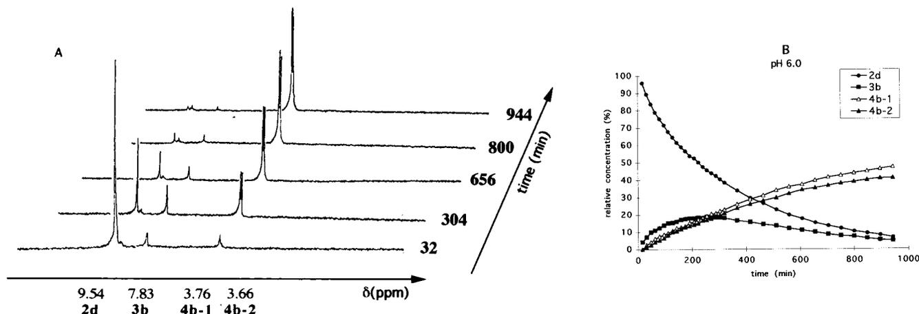
**Figure 6.** Stack plot of  $^{31}\text{P}$  NMR spectra recorded during hydrolysis of the phosphoramidic acid monoester **2d** in cacodylate buffer at pH 6.0, 25 °C (A). Corresponding  $^{31}\text{P}$  NMR time course (B).
