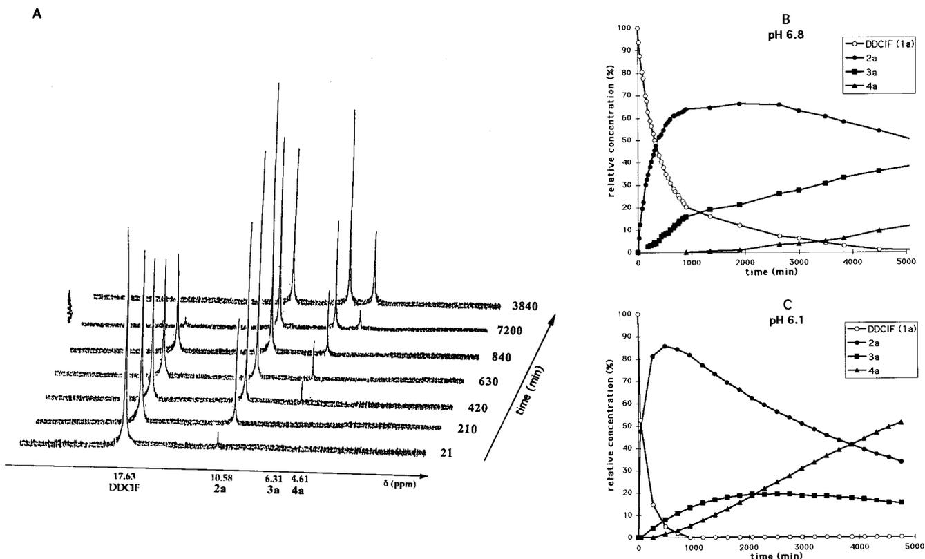
**Figure 2.** Stack plot of  $^{31}\text{P}$  NMR spectra recorded during DDCIF (**1a**) hydrolysis in 0.1 M cacodylate buffer at pH 6.8, 25 °C (A).  $^{31}\text{P}$  NMR time course at pH 6.8 (B) and 6.1 (C).
