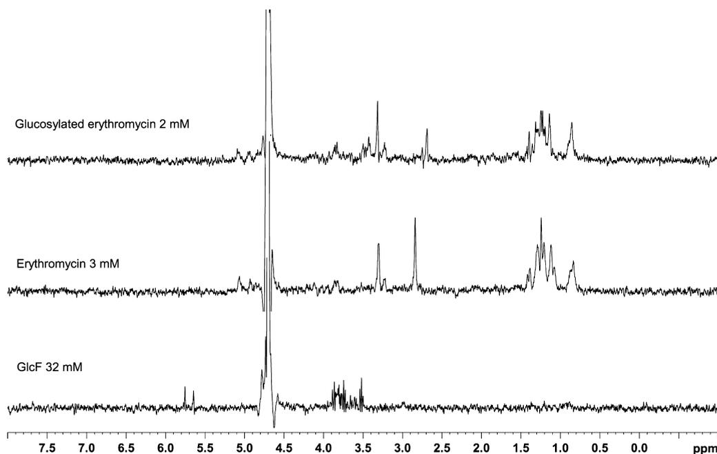
**Figure 7.**  $^1\text{H}$  STD-NMR spectra (500 MHz) of EryBI D257G (0.1 mM) and substrates and product in deuterated phosphate-buffered saline (50 mM, pD 7.6).
