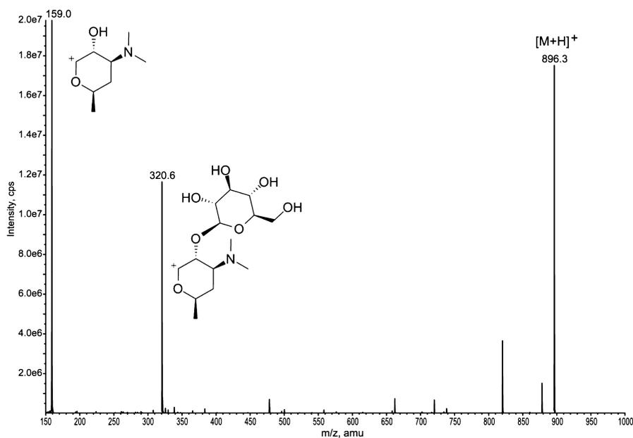
**Figure 4.** Electrospray tandem MS/MS spectrum of glucosylated erythromycin and fragmentation demonstrating the regioselective nature of glucosylation. The spectrum was recorded on an Applied Biosystems 2000Qtrap instrument in positive mode. The configuration of the glycosidic linkage was determined by <sup>1</sup>H NMR analysis.
