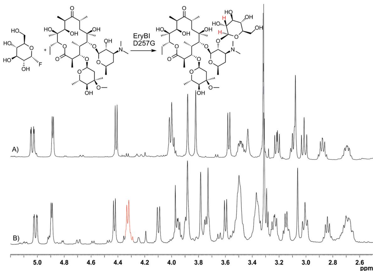
**Figure 5.**  $^1\text{H}$  NMR spectrum (500 MHz) ( $\text{CDCl}_3$ ) of (A) commercial erythromycin and (B) the glycosynthase product (glycosylated erythromycin). The glucosyl anomeric proton is highlighted at 4.32 ppm. The  $^3J_{\text{H}_1,\text{H}_2} = 8$  Hz coupling indicates a  $\beta$ -glycosidic linkage.
