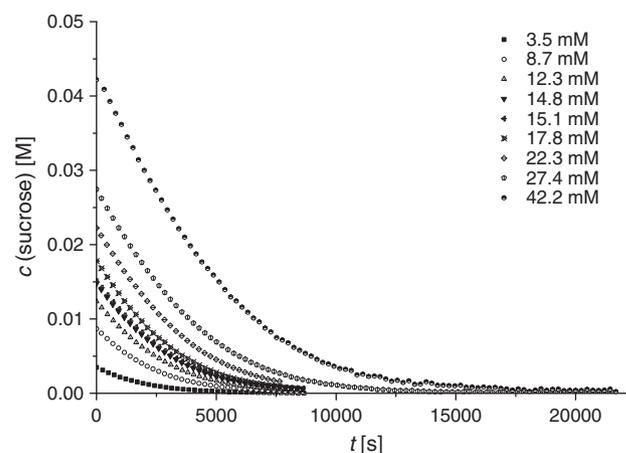
**Fig. 1.** Overview of progress curves recorded for the hydrolysis of sucrose by invertase. Initial concentrations of sucrose are listed in the legend (every second data point is shown).
