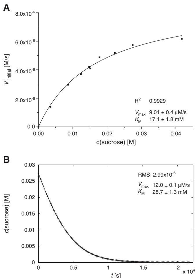
**Fig. 3.** Determination of  $K_m$  and  $V_{max}$ . **A:** Michaelis–Menten plot of invertase reaction derived from initial velocities of each progress curve. The fit afforded  $K_m = 17 \text{ mM}$  and  $V_{max} = 9 \mu\text{M/s}$ . **B:** Progress curve analysis of invertase reaction with initial sucrose concentration of 27.4 mM. The data was fitted according to Eq. (1) and yielded  $K_m = 29 \text{ mM}$  and  $V_{max} = 12 \mu\text{M/s}$ .
