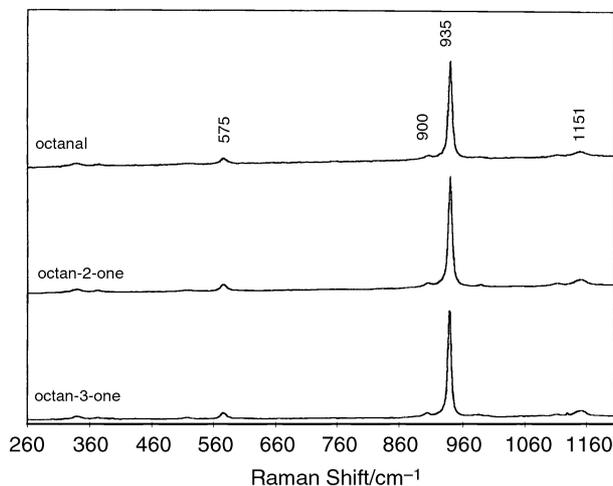
**Fig. 6** The Raman spectra of VPD precursors prepared using aldehydes and ketones as reducing agents.
