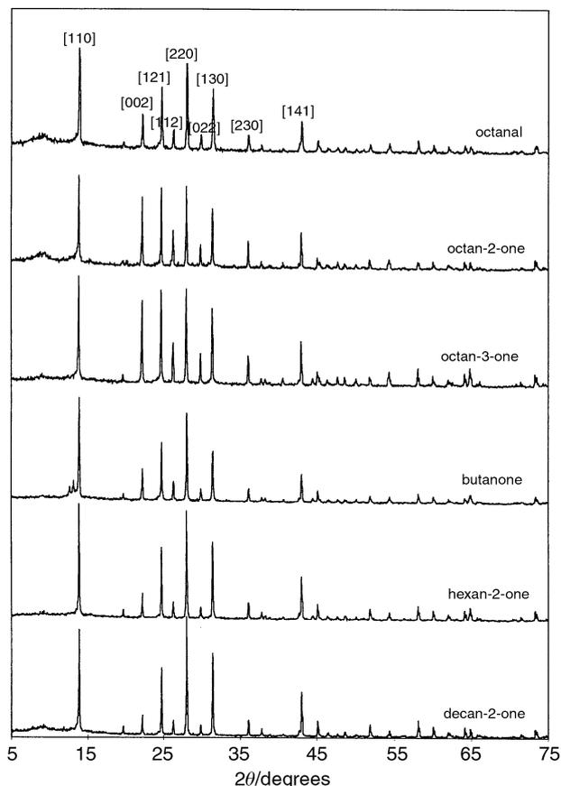
**Fig. 1** Powder XRD patterns of VPO precursors prepared using aldehydes and ketones as reducing agents. The pattern is indexed to the reflexions for  $\text{VO}(\text{H}_2\text{PO}_4)_2$ .
