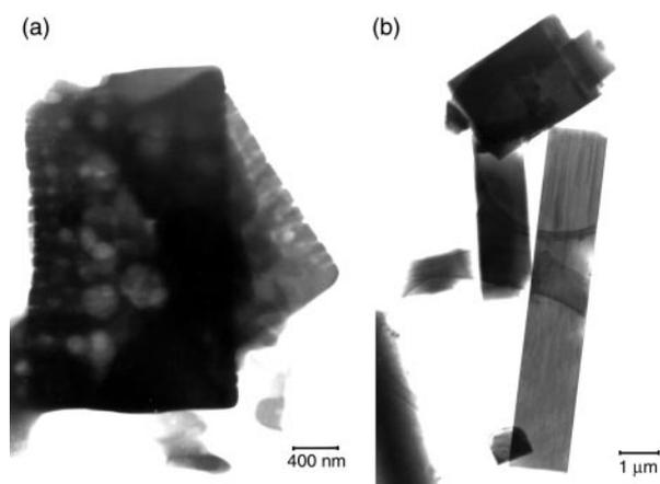
**Fig. 4** Bright field transmission electron micrographs for  $\text{VO}(\text{H}_2\text{PO}_4)_2$ . (a)  $\text{VOPO}_4 \cdot 2\text{H}_2\text{O}$  and octan-3-ol, (b) VPO method with octan-2-one.
