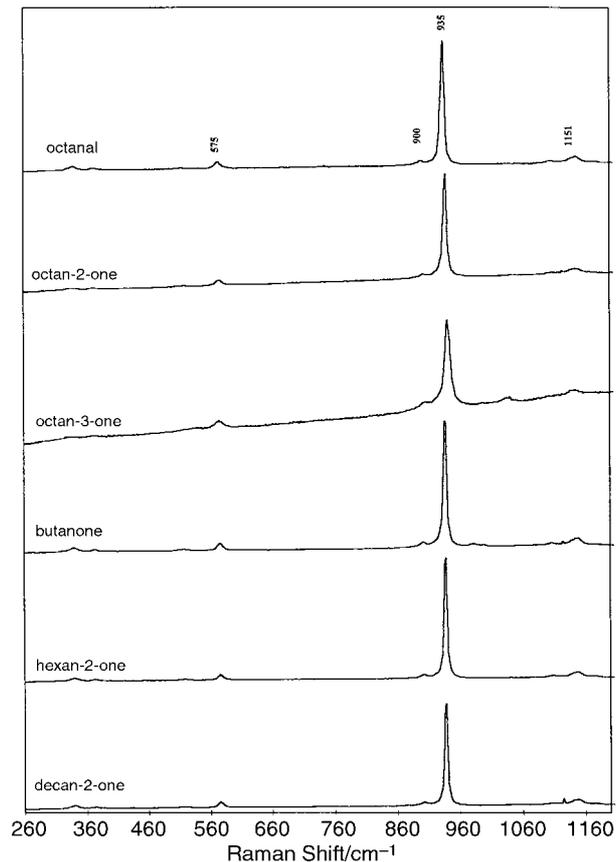
**Fig. 2** Raman spectra of VPO precursors prepared using aldehydes and ketones as reducing agents.
