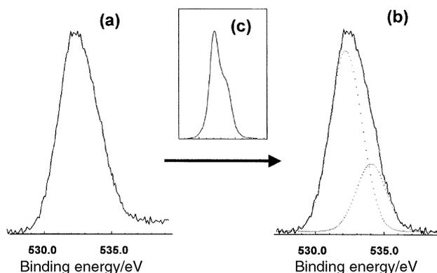
Fig. 12 Illustration of the analysis procedure applied to the O(1s) spectra from the catalysts derived from  $VO(H_2PO_4)_2$ . The raw spectrum (a) is subjected to a non-linear background removal procedure followed by curve-fitting (curve (b)), making use of the deconvoluted profile (c) both to confirm the existence of 2 spectral components and to estimate component parameters.
