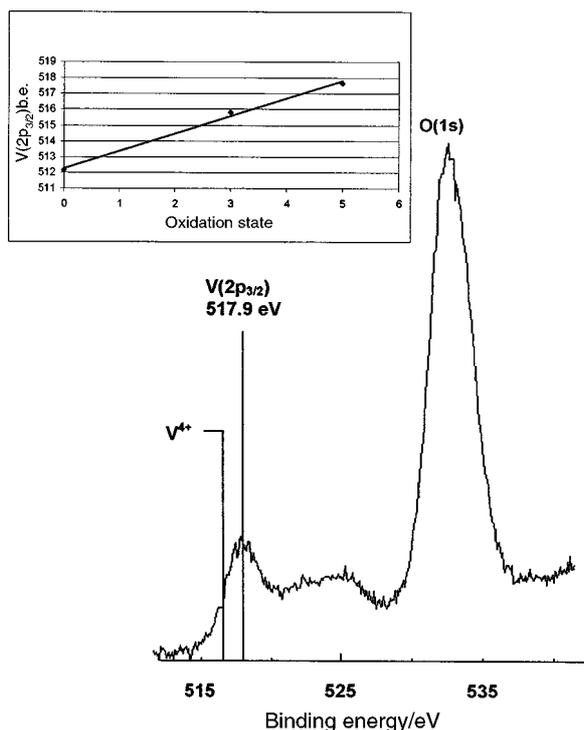
Fig. 11 V(2p) + O(1s) spectral region for the sample corresponding to the curve-fit in Fig. 12. The binding energy scale has been charge-corrected relative to a C(1s) binding energy of 285.0 eV. The expected binding energy position for  $V^{4+}$  species is estimated from the plot of V(2p<sub>3/2</sub>) binding energy vs. oxidation state shown inset (data from ref. 19), and is indicated on the spectrum.
