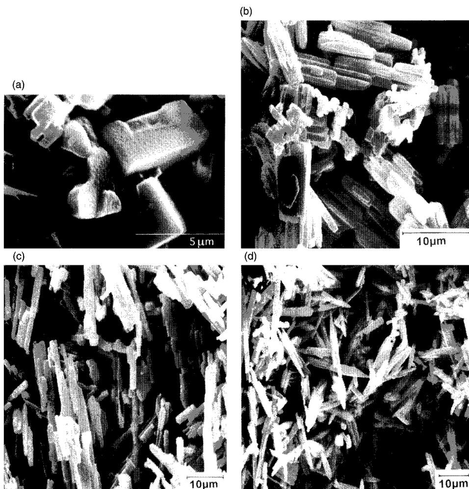
**Fig. 3** SEM micrographs of  $\text{VO}(\text{H}_2\text{PO}_4)_2$ . (a)  $\text{VOPO}_4 \cdot 2\text{H}_2\text{O}$  and octan-3-ol, (b) VPO method with octanal, (c) VPO method with octan-2-one, (d) VPO method with octan-3-one.
