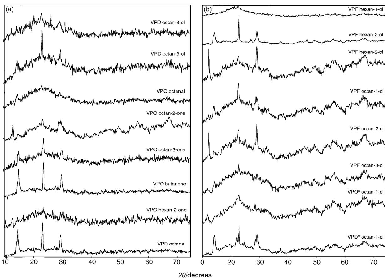
**Fig. 9** Powder XRD patterns of catalysts after reaction.
