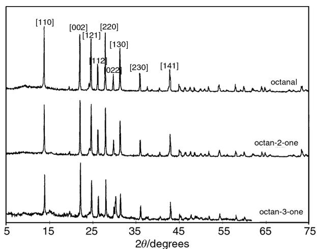
**Fig. 5** Powder XRD patterns of VPD precursors prepared using octanal, octan-2-one and octan-3-one.
