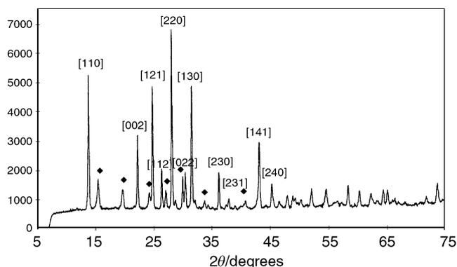
**Fig. 8** Powder XRD pattern of the product of reduction of  $\gamma$ -VOPO<sub>4</sub> with isobutanol, (◆) denotes lines attributed to VOHPO<sub>4</sub> · 0.5H<sub>2</sub>O.
