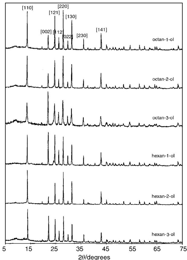
**Fig. 7** Powder XRD patterns for  $\text{VO}(\text{H}_2\text{PO}_4)_2$  prepared by alcohol reduction of "anhydrous  $\text{VOPO}_4$ ".
