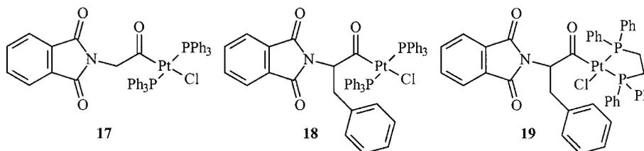
bis(diphenylphosphanyl)ethane complex **19** was synthesised from **18** by ligand exchange.
