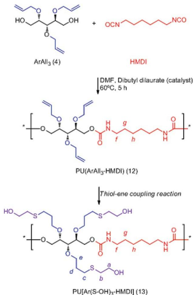
**SCHEME 3** Polymerization reaction of compound **4** with HMDI and subsequent thiol-ene coupling reaction with 2-mercaptoethanol. [Color figure can be viewed in the online issue, which is available at [wileyonlinelibrary.com](http://wileyonlinelibrary.com).]
