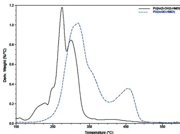
**FIGURE 2** Comparative curves of thermal degradations under inert atmosphere of PU(ArAll<sub>3</sub>-HMDI) and PU[Ar(S-OH)<sub>3</sub>-HMDI] homopolymers. [Color figure can be viewed in the online issue, which is available at [wileyonlinelibrary.com](http://wileyonlinelibrary.com).]
