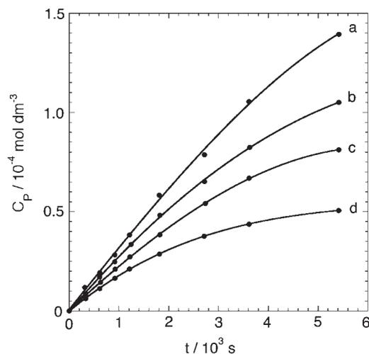
Fig. 8. Time dependence of concentration of produced 4-nitrophenol catalyzed by free phosphatase for the initial substrate concentration of  $5 \times 10^{-4} \text{ mol dm}^{-3}$  (a),  $2 \times 10^{-4} \text{ mol dm}^{-3}$  (b),  $1 \times 10^{-4} \text{ mol dm}^{-3}$  (c), and  $8 \times 10^{-5} \text{ mol dm}^{-3}$  (d). The pH of the solution was 4.8.
